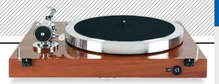
ABOVE: The C-Note arm's counterweight is damped by a sorbothane-like polymer while the nylon thread for the bias outrigger sits in a groove around the arm base, improving stability. The tonearm leads connect via a five-pin SME/DIN connector
